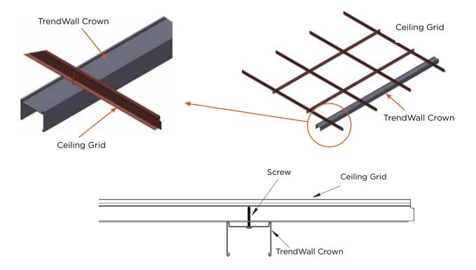
Armstrong Silhouette ceiling requires the use of Grid Clips to attach the Crown to the grid, available for order from Trendway (Special part number 404765). Caddy Clips may be used to attach the Crown to many ceiling grids. Use one every 2' of Crown. **Caution:** There will be a loss of 1/2" to 5/8" ceiling height adjustment when using Caddy Clips.
