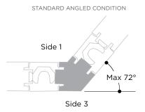
**3-Way Conditions** | **3-Way Conditions, commonly called "T" conditions,** are used to create a **3-way panel connection in panel runs.** They can be ordered with electrical punch-outs to accommodate either hardwire or modular power. Punch-Outs are available on the outside face only.
