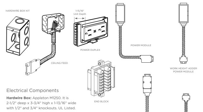
**Ceiling Feed:** Supplies power from the ceiling to the distribution block on the Power Module. Length is 12' of conduit with 13' of wire.
