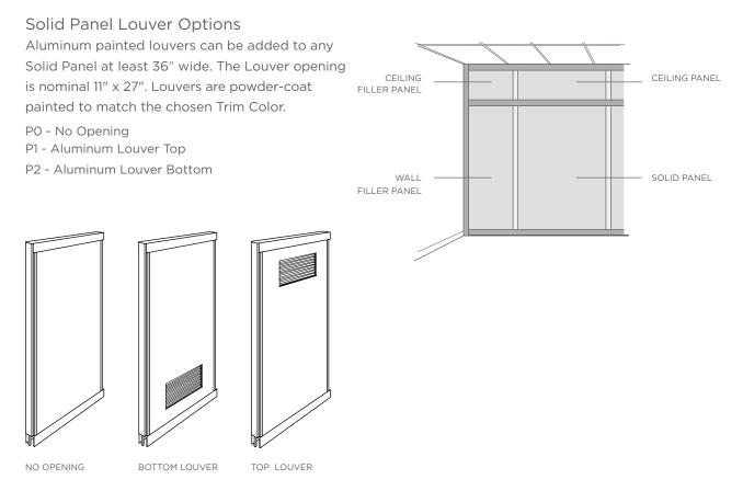
Filler Panels | Filler panels are installed at the end of a panel run that meets a fixed wall. They accommodate window mullions, moldings, uneven wall conditions and irregular shaped conditions. Available
